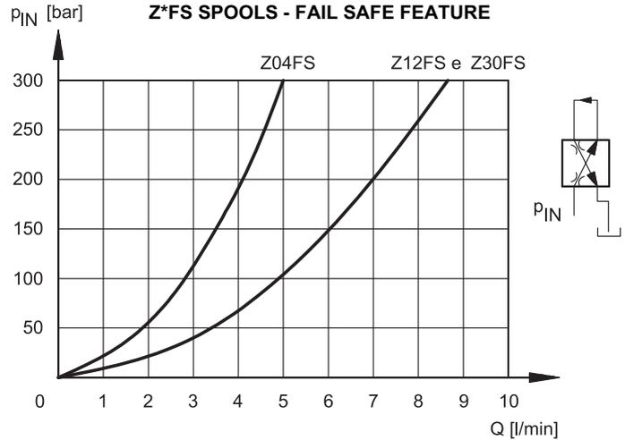
Flow  $P \rightarrow B / A \rightarrow T$  with valve in fail safe position, depending on the incoming pressure.
