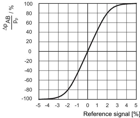
The diagram shows the valve pressure gain, expressed as % of the ratio between the port pressure variation in A or B ( $\Delta p_{AB}$ ) and the P system pressure, according to the reference signal.
