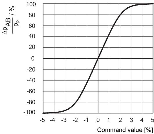
The diagram shows the valve pressure gain, expressed as % of the ratio between the port pressure variation in A or B ( $\Delta p_{AB}$ ) and the P system pressure, according to the reference signal. In practice, the pressure gain states the valve reaction towards external disturbances aimed at changing the actuator position.
