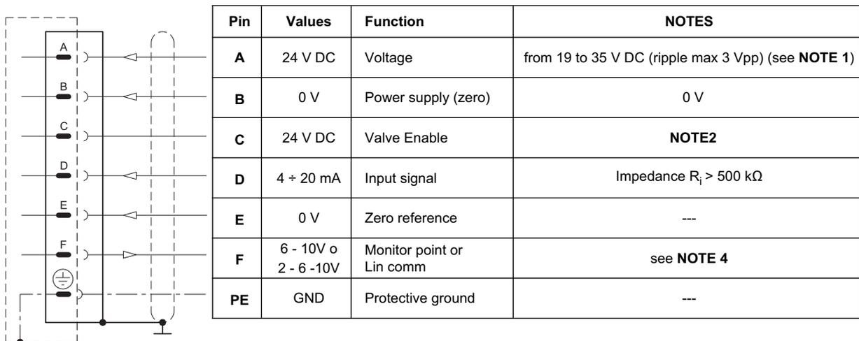
**NOTE 1:** preview on the Pin A (24 VDC) an external fuse for protecting electronics. Fuse characteristics: 5A/50V type fast.
