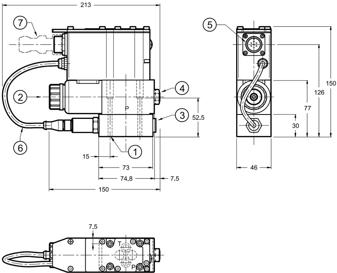
**NOTE:** at the first start up, or after a long period of no use, it is necessary to vent the air through the breather (2) placed at the end of the solenoid tube.
