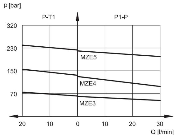
The curves have been obtained with inlet pressure 50 bar greater than nominal pressure. Pressure values in P1 greater than 50 bar reduce flow values considerably.
