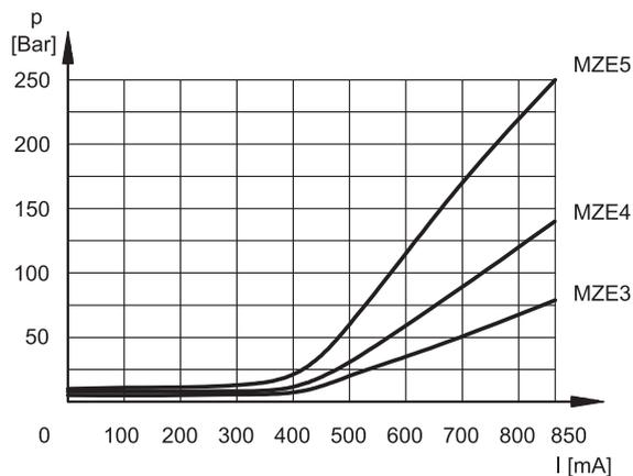
The curves have been obtained with working lines closed (without flow).
