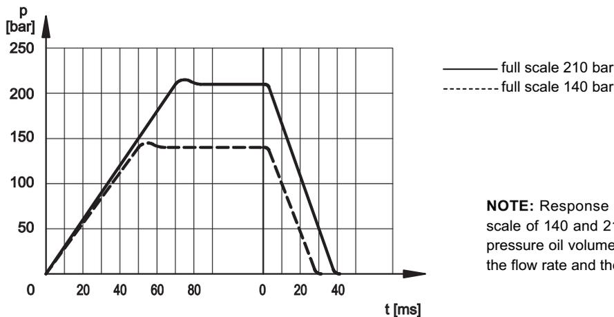
**NOTE:** Response times are obtained by using valves with a full scale of 140 and 210 bar, with an input flow rate of 10 l/min and a pressure oil volume of 0,5 lt. The response time is affected both by the flow rate and the oil volume in the pipework.
