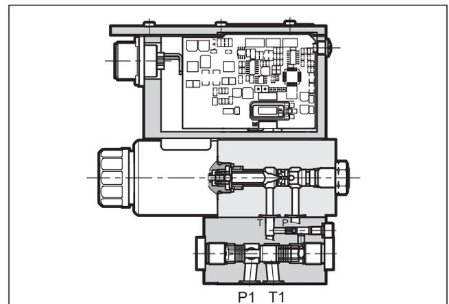
— The PRE3G valve is a pilot operated pressure control valve with integrated electric proportional control and mounting interface in compliance with ISO 4401 (CETOP RP 121H) standards, controlled directly by an integrated digital amplifier (see par. 4).
