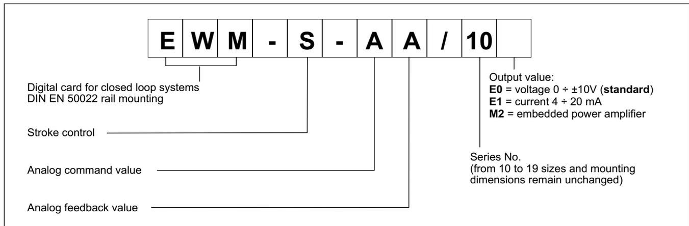
This module supports the simple point-to-point positioning with hydraulic drives. The deceleration characteristics can be defined with the command CTRL, choosing between linear (LIN) or nearly square root (SQRT1) parameters. See at par. 4, adjustments.
