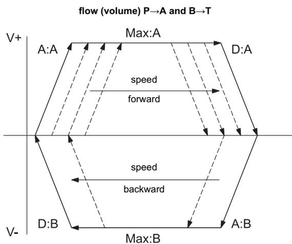
The actuator position is measured by an analog transducer and compared with a specified target position. The target position is adjusted with an external potentiometer or preset by an analog input from an external controller (PLC). It's possible to define the axis speed also by an external command speed.
